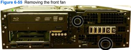
Pull the assembly toward the rear of the unit, and then lift it out of the chassis. 7.
